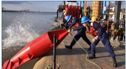
Two Coast Guardsmen prepare to release a red nun buoy used to mark the outer limits of a navigation channel.
