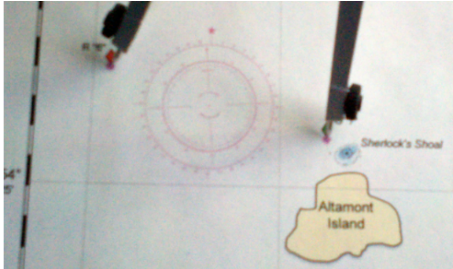
Figure 2.6. Placing the dividers on two points.
