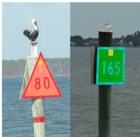
Figure 1.21. Intracoastal waterway day markers. (Note the yellow markers to indicate that these apply to the ICW.)
